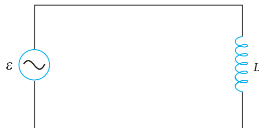
FIGURE 7.5 An ac source connected to an inductor.
